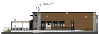
Proposed west elevation includes changing the façade to cedar lap sidings in place of painted EIFS. Two vertical corrugated rustic metal panels will be added at both ends of the façade. Two doors are proposed one serving the entrance for customer and other leading to shared area of suites. The number of windows is reduced. Entire faced will be capped with firestone matt black color.
